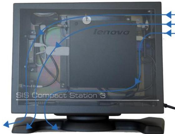
A USB powered fan is used to ventilate the PC inside the enclosure. The air is aspirated on the top side and pushed out through the bottom ventilation grid. The fan stops when the PC is powered off.
