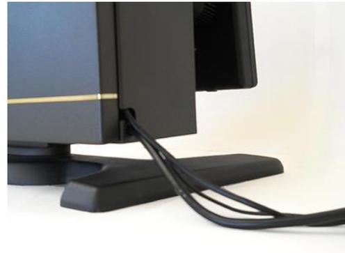
The SIS CS The SIS-CS 3 has a multi format flash memory card reader exposed to the operator. The keyboard, mouse and even the power cable are all connected inside the enclosure. When closed these peripherals cannot be disconnected. The monitor cables are clamp-in and neatly tucked away once the monitor mount is in place.
