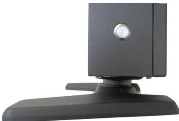
Computer manufactures generally seal the PC allowing only authorized brand technicians to access to the internal component. To avoid being in conflict with the product warranty the SIS Compact Station power button was designed to be non-intrusive. The PC is switched on mechanically with an external push button and internal cable system.
