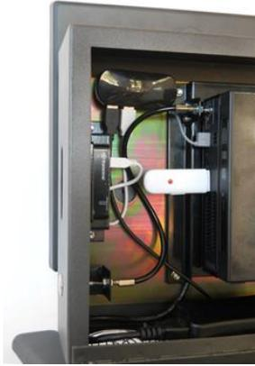
The secure enclosure typically have a 3G/4G modem installed enabling access to mobile networks.
