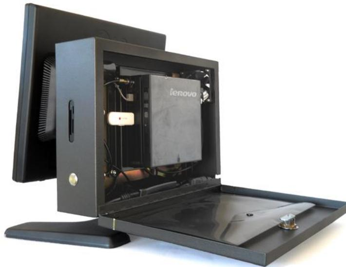
The SIS CS is supplied with the latest ultra small form factor PC technology. With reliability being the key factor the PC The design supports a standard VESA mountable small form factor PC. with the choice of the processing power of an Intel core i3 to i7. When opened, the enclosure is designed to expose all computer hardware and peripherals attached making it simple to maintain..
